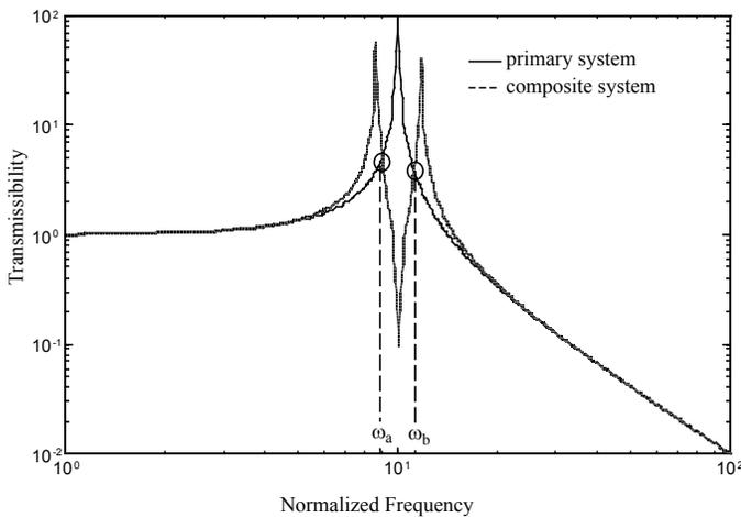
**Figure 3. Transmissibility curves of a single degree-of-freedom primary system and the coupled system with a TVA tuned to the resonance of the primary system. Encircled intersections are invariant to TVA damping.**
