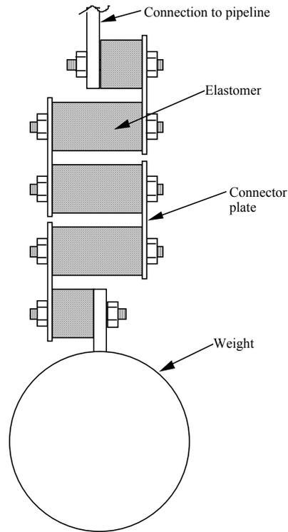
**Figure 6. The TVA configuration for the arctic pipeline (early configuration; from Hart, et. al., 1993).**
