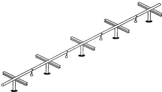
Early TVA configurations on Arctic Pipelines consisted of masses suspended by elastomeric springs dangling below the pipeline. The TVAs used in this application have reduced the
