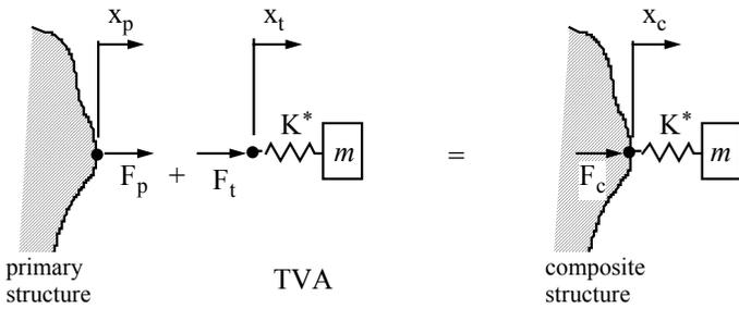
**Figure 1. Impedance coupling of a TVA to a primary structure in the direction of the defined coordinates.**
