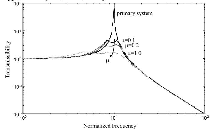
**Figure 4. Transmissibility curves of a single degree-of-freedom primary system and the coupled system with a TVA designed with the equal-peak method. Three mass ratios are shown for the coupled system.**
