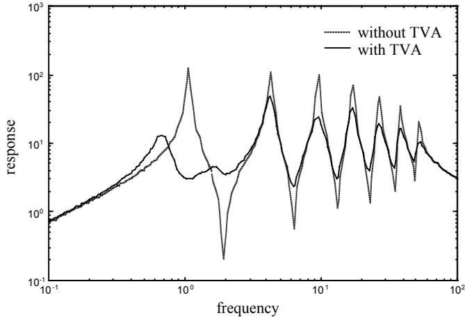
**Figure 2. The effect of a TVA on the broadband response of a continuous structure. The TVA mass is 5% of the structural mass and is tuned to the first mode of the structure. The structure has 3% damping and the TVA has 20% damping.**
