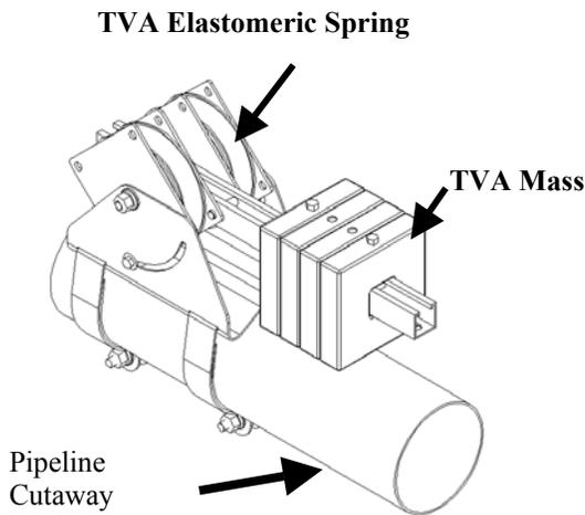
**Figure 7. The TVA configuration for the arctic pipeline (above pipeline configuration).**
